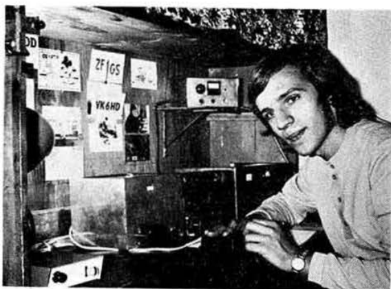
Martin Kumpost, OK1MCW ex-OL5ANJ , specializes in low power 160m working. His equipment consists of (l to r) HM1C electronic keyer, 160m converter, W-10-L receiver and HM10W transmitter. W1BB photograph
